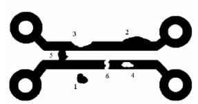
Fig. 1 - Example of a PCB layout defects:
